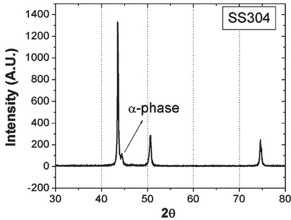
Fig. 6. XRD pattern of an SS304 surface nitrided in pure  $N_2$ , showing the induced  $\alpha$  phase shifted to the right of the  $\gamma$  peak (intensity given in arbitrary units and  $2\theta$  angle in degrees).
