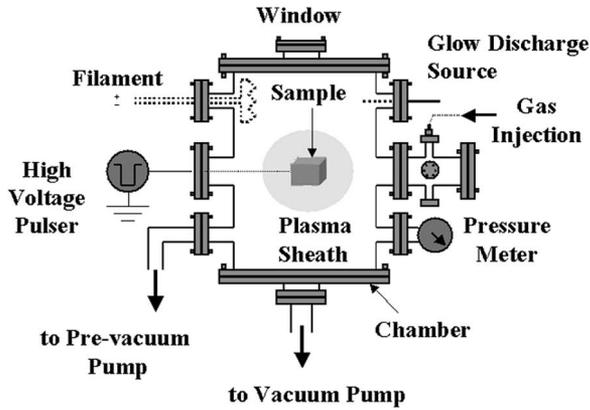
Fig. 4. Experimental setup used for the PIII system.
