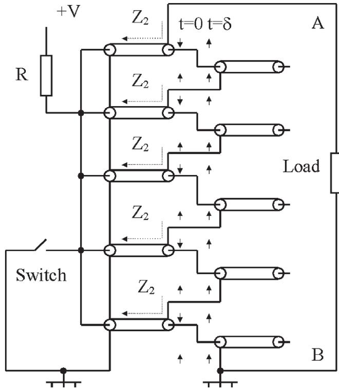
Fig. 1. Blumlein pulser made of ten coaxial lines.
